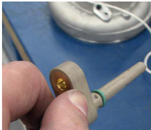
Figure 68: Lubricate O-Ring, Install, Check Depth, and Tighten Bolt
