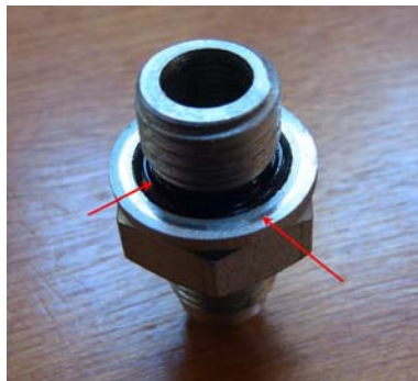
Figure 77: Oil Inlet Fitting With O-Ring and Washer (sealing contact on washer can be seen)
