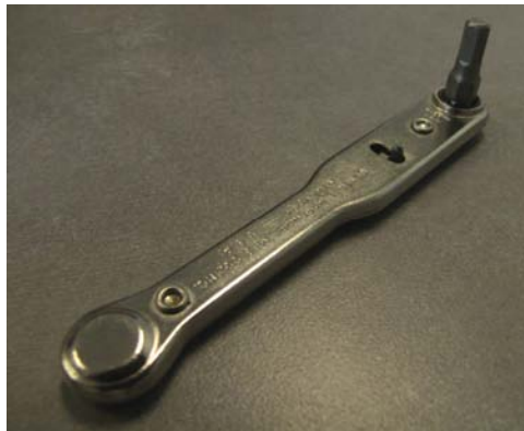
Figure 75: This is a Better Tool For Tightening the WG Bracket Bolts
