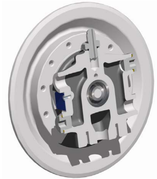
Figure 102: Oil and Water Cavity Detail
