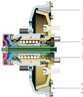
Powerwedge liner provides consistent performance throughout the life of the product, and provides for smoother engagement, reducing stress in belts and other components.
