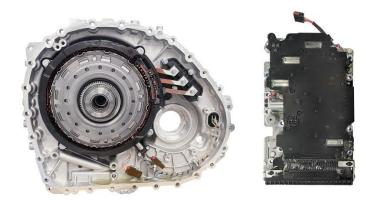
BorgWarner supplies next-generation triple-clutch P2 drive module to HYCET Transmission (The housing is designed and provided by HYCET)
