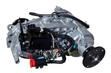
BorgWarner's part-time AWD transfer case features the company's state-of-the-art electronic shift-on-the-fly technology to deliver quick, smooth shifts between two-wheel and all-wheel drive at the turn of a dial.
