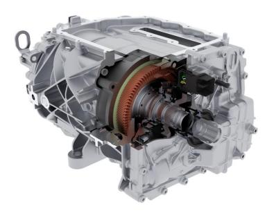
BorgWarner's High Voltage Hairpin (HVH) 320 motor capable of 97% peak efficiency and equipped with 800-volt capabilities
