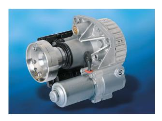
BorgWarner's state-of-the-art GenV AWD coupling provides Volvo's XC90 with high torque accuracy, improved handling and stability for a fun-to-drive experience.
