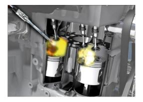
BorgWarner BERU Systems has delivered over three million pressure sensor glow plugs (PSGs) to diesel automakers and aftermarket customers around the world. PSGs combine a highly efficient glow plug to improve diesel engine cold starts with an integrated pressure sensor to improve engine efficiency.
